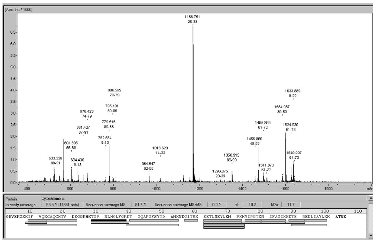
Fig. 2. Analysis of cytochrome C peptides digest (850 fmol/ $\mu$ l) by MALDI-Tof-MS. In the mass spectrum, each ion has been labeled by both the monoisotopic mass and the amino-acid position in the protein sequence. The bottom of the figure depicts the protein sequence coverage after database searching.
