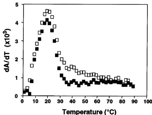
FIGURE 3: UV melting derivative curves for AC-oligo ( $7.5 \mu\text{M}$ ) at  $260$  nm (solid squares) and  $268$  nm (open squares). First derivative curves of the melting profiles shown in Figure 2 are monophasic at all wavelengths.
