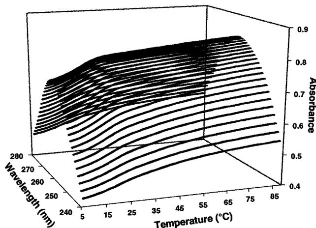
FIGURE 2: Absorbance as a function of temperature at several wavelengths for AC-oligo ( $7.5 \mu\text{M}$ ). UV spectra were collected from  $310$  to  $218$  nm every  $2^\circ\text{C}$  from  $0$  to  $89^\circ\text{C}$ . For clarity, only data from  $240$  through  $280$  nm are shown. UV detects only the low-temperature transition at all wavelengths.
