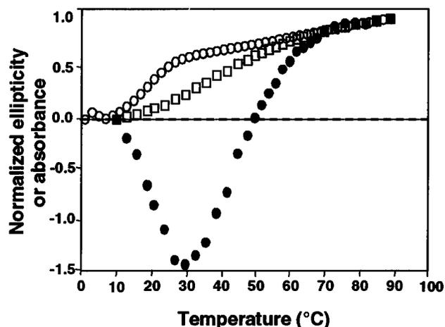
FIGURE 1: Normalized  $A_{260}$  (open circles),  $\theta_{253}$  (squares), and  $\theta_{263}$  (solid circles) as a function of temperature for AC-oligo ( $7.5 \mu\text{M}$  strand).  $A_{260}$  and  $\theta_{253}$  detect different transitions. The low-temperature transition detected by  $\theta_{263}$  corresponds to the  $A_{260}$  transition. The high-temperature transition detected by  $\theta_{263}$  corresponds to the  $\theta_{253}$  transition.
