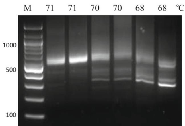
Fig. 5. Analytical gel (2% agarose) of replicate dsDNA “stitching” PCRs. Two double-stranded DNA fragments (190 and 480 bp, previously synthesized by R-PCR), containing a single 17 nucleotide overlapping region, amplified over a range of annealing temperatures: *lanes 2–3* (71°C), *lanes 4–5* (70°C), *lanes 6–7* (68°C). *Lanes 2* and *3* illustrate successful amplification of the ~650 bp target.
